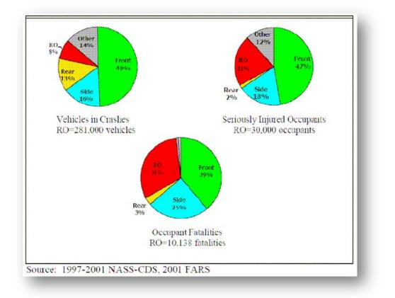
Figure 1.1: The percentage of rollover accident compared with the others type of accidents. (Source: NASS-CDS, (2001))
