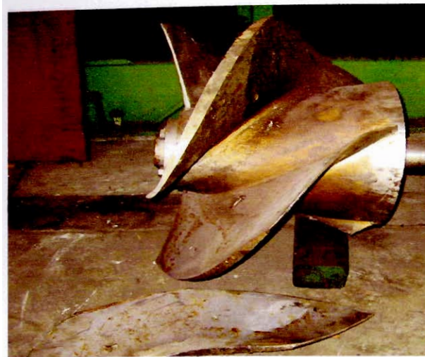
Figure 1.1: The failure mode of a sheared blade at the root of the impeller (Source: Industry, Dec 2003)
