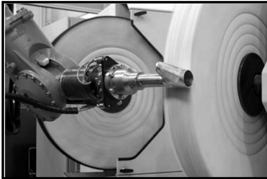
Figure 2.3: Robot Aided Polishing in the Sanitary Fitting Industry
