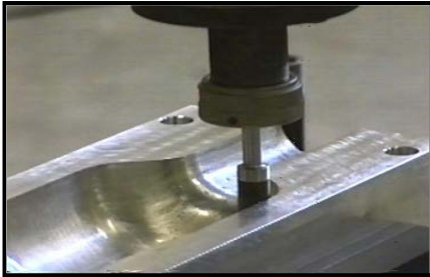
Figure 2.1: Polishing Scene of a PET Bottle Mold
