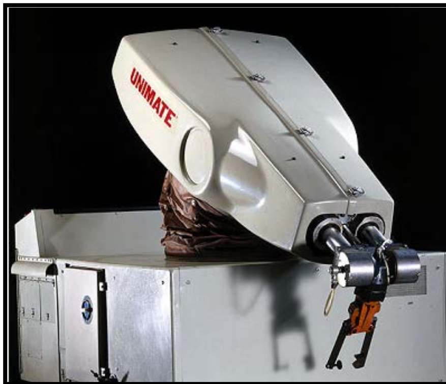
Figure 2.4: The First Industrial Robot by Unimation Inc.
