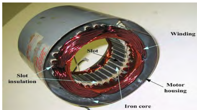
Figure 2.2: Stator of the AC induction motor
