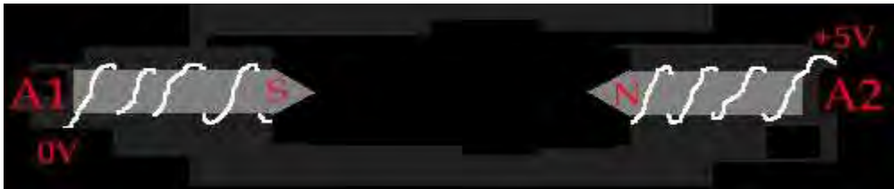
Figure 2.4 The opposite poles created when the signal is reversed
