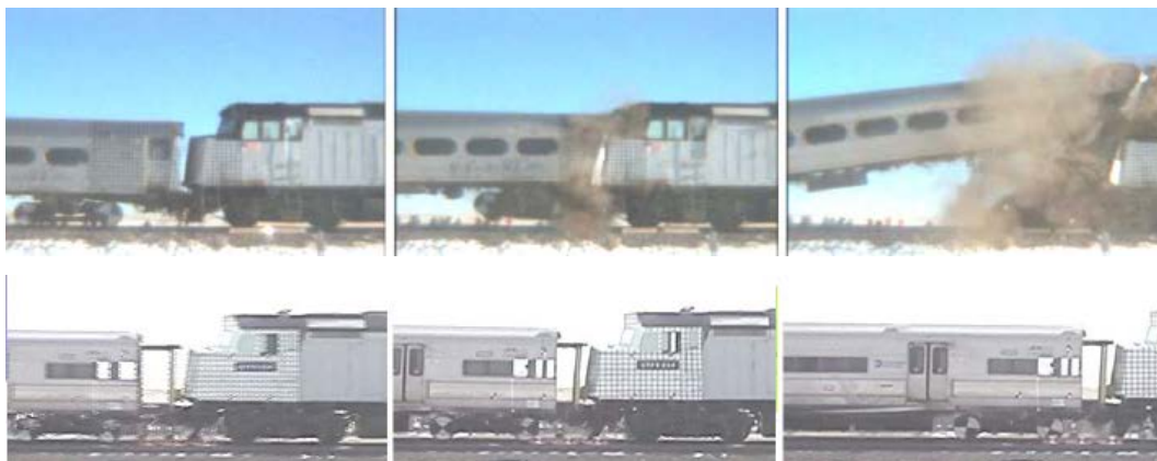
Figure 2.1: Frames from Train-to-Train Test Movies of Conventional and CEM Equipment [2].
