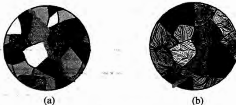
Figure 2.1: Types of crack; (a) Intergranular Crack (b) Transgranular Crack
