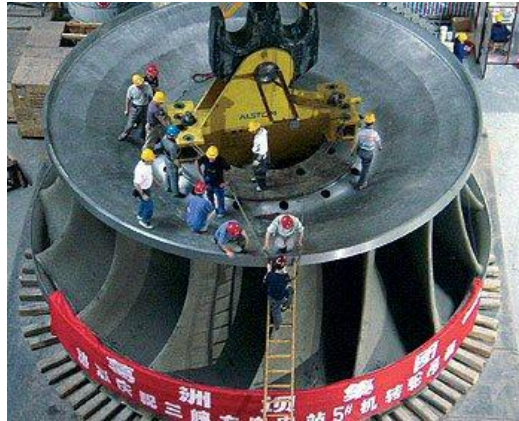
Figure 1.2: Hydro Turbines of three Gorges Dams in Construction (Source: http://www.trelleborg.com/ )
