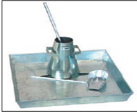
Figure 2.1: Apparatus set for slump test
