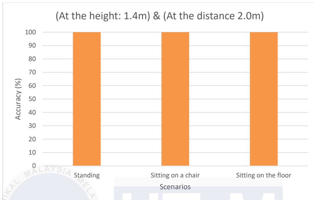
Figure 4.9 Graph of Fall Detection Accuracy to Differ Non-Fall Postures
