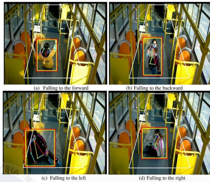
Figure 2.21 The detection results of fall in different directions [28].
