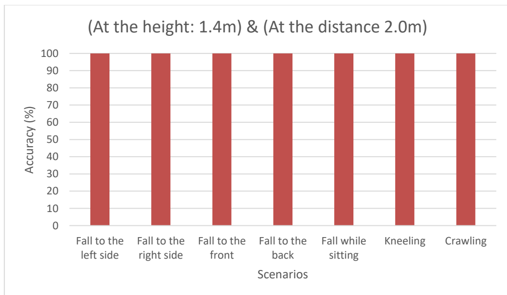
Figure 4.5 Graph of Fall Detection Accuracy for Different Fall Postures
