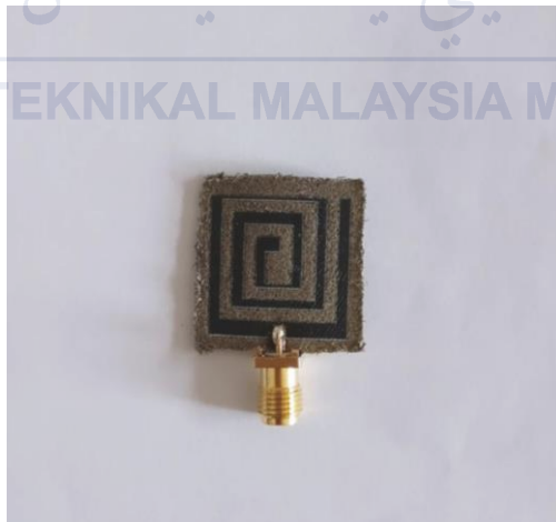
Figure 3.25: Graphene antenna soldered with SMA connector.
