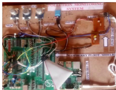
Figure 2.17: Hardware Setup of Raspberry-Pi
