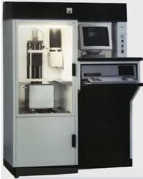
Figure 2.14 SLA-1, the first commercial prototyping device from 3D Systems
