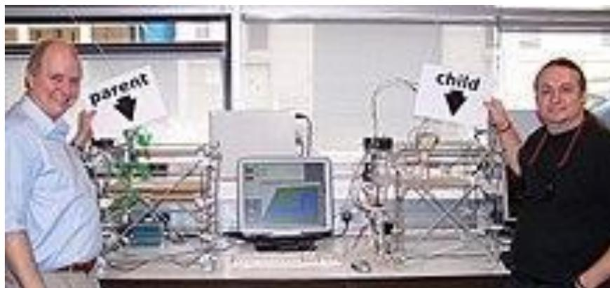
Figure 2.15 The machine on the left produced all the plastic parts for the machine on the right. Adrian Bowyer (left) and Vik Olliver (right) are members of the RepRap project.
