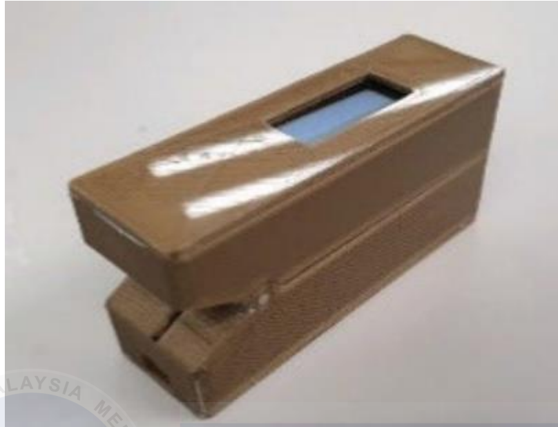
Figure 2.2 Finger clip used for measure.
