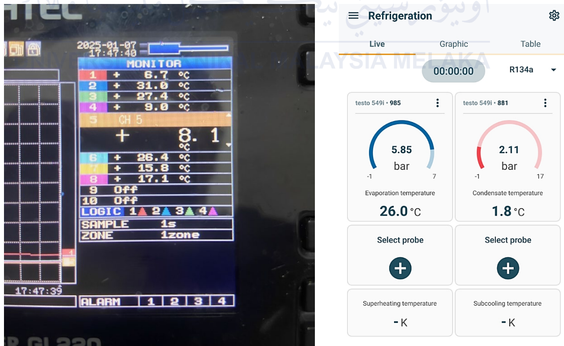
Figure 4.2 Display value for each data point in temperature result on data logger and pressure results on Testo Smart app
