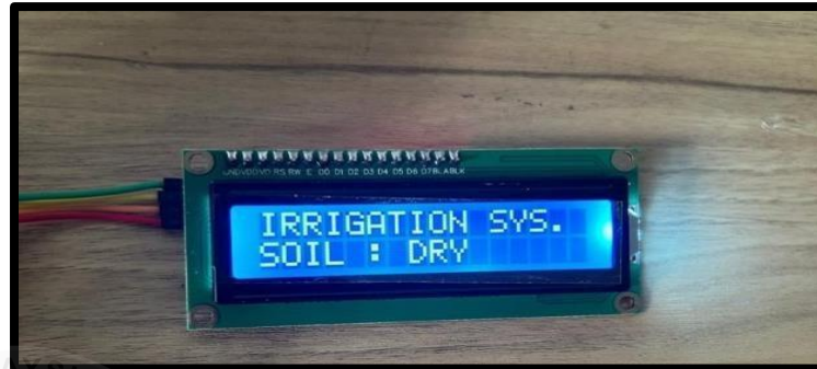
Figure 4.3 LCD display Dry Conditions
