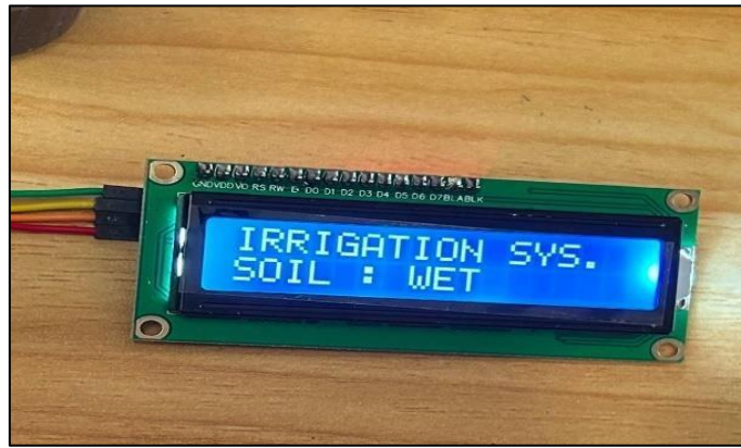
Figure 4.5 LCD Display Wet Conditions
