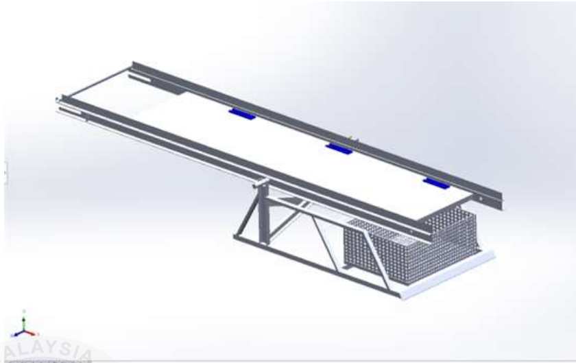
Figure 4.2 Trash Collector Conveyor device
