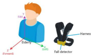
Figure 2.2 The prototype design with sensing axes of MPU6050 on the chest of the person[12]
