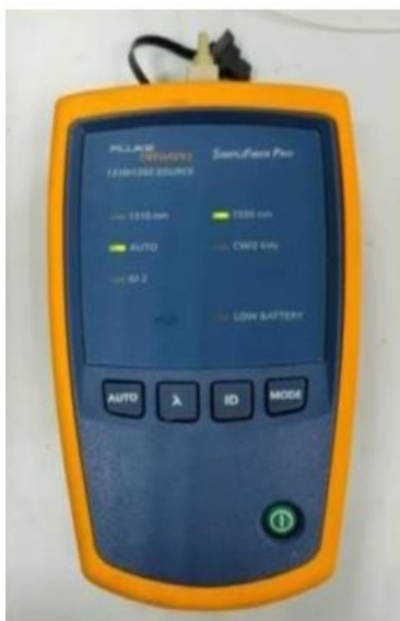
Figure 3.7: The light source that transmits 1350nm and 1550nm light
