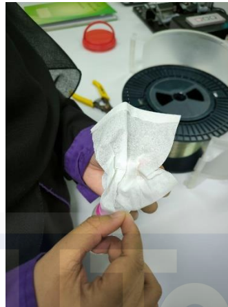
Figure 3.12: Fiber being cleaned with isophrophyl alcohol
