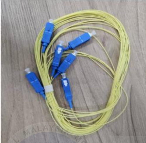
Figure 3.1: SC/UPC connectors for single mode fiber pigtails
