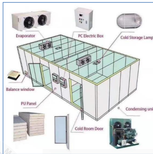
Figure 2.5 Requirements to choose a cold room
