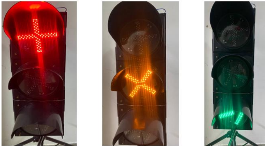
Figure 32 – Red, Yellow and Green LED Traffic Light
