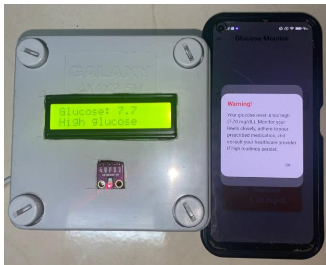
Figure 4.12: When blood glucose level is in high range, there is a warning notification.
