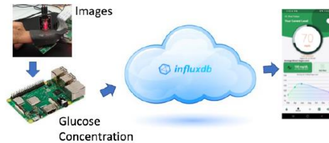
Figure 2.7 Overview of the proposed non-invasive blood glucose monitoring system[18].
