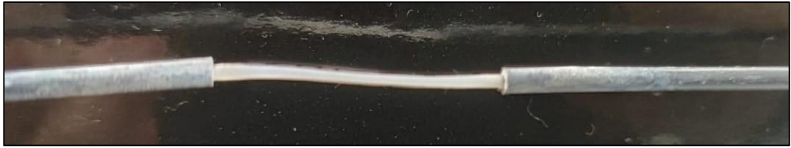
Figure 3.34: 4cm expose fiber with zinc oxide coated.
