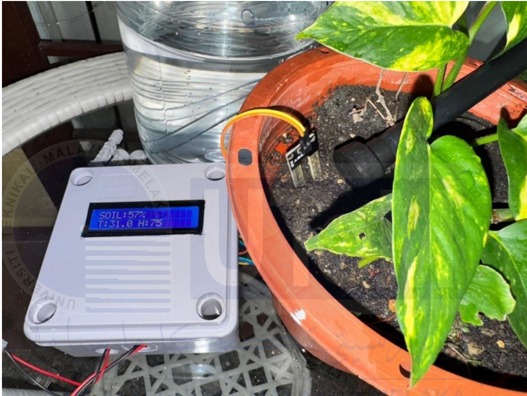
Figure 4.2 The irrigation stops once the soil moisture exceeds the threshold.
