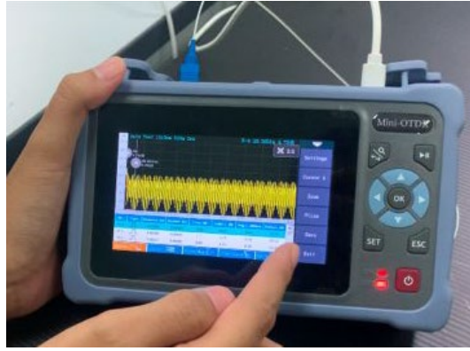
Figure 3.21 Output power measured using OTDR
