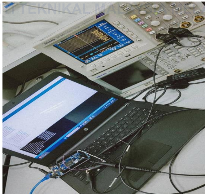
Figure 3.29: Connection of microcontroller and oscilloscope for SPWM signal generation
