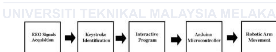
Figure 2. 12 Block diagram of BCI robotic arm
