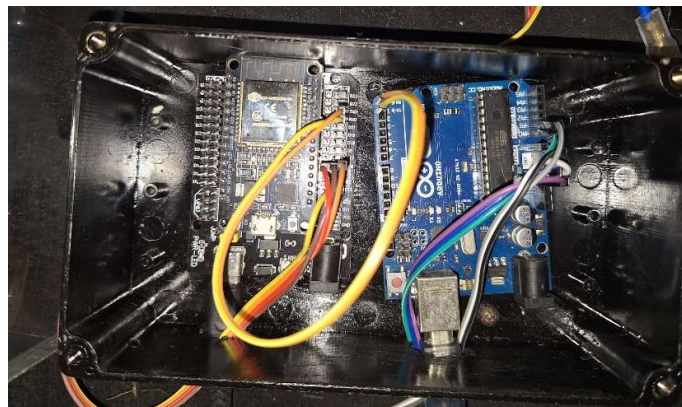
Figure 4.12: Connection between Arduino Uno and ESP32.
