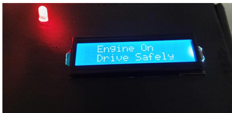
Figure 4.15 LCD and LED when the engine successfully turns on
