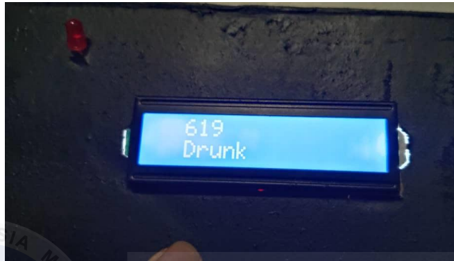
Figure 4.16 LCD when the reading indicates drunk
