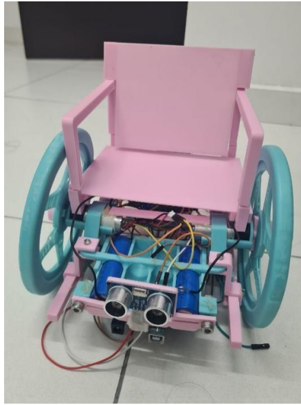
Figure 3.36 Sensor 1 placed on the front of wheelchair
