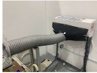
1hp air conditioner is supported by a custom-made flexible round duct to direct the cool air towards the chamber.
