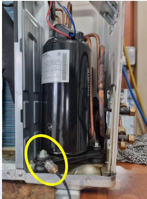
Figure 4.2 Vibration sensor at the bottom of compressor (near to mounting)
