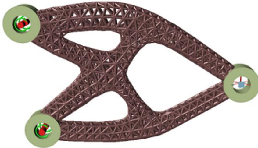
Figure 3.9 Result after LSO in Altair Software (Lattice Optimization, n.d.)
