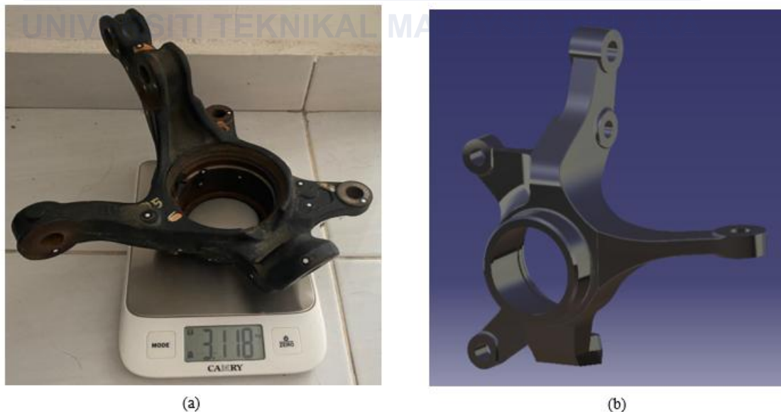
Figure 3.20 : (a) Actual Steering Knuckle (b) Base Model
