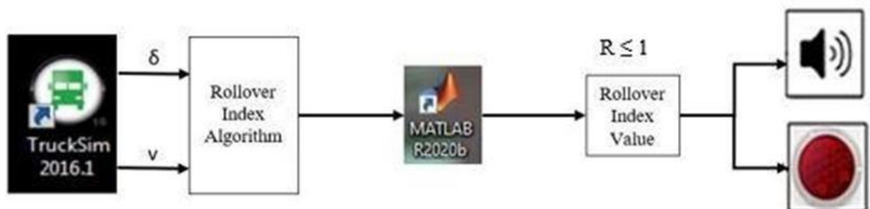
Figure 3. 4 Input from Algorithms in Software in the Loop
