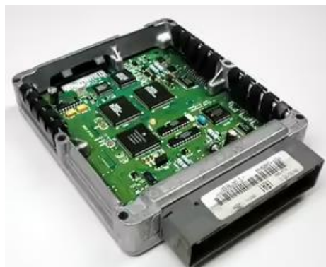
Figure 2.22 Modern Electronic Control Unit(ECU) (Karim Nice, 2021)
