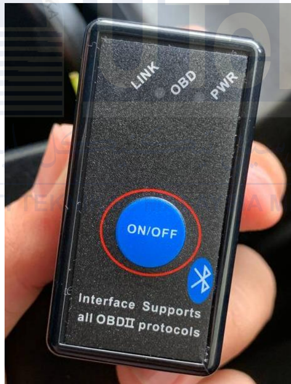
Figure 3.3 An OBD-II Wireless Adapter
