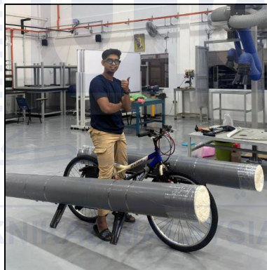
Figure 4.2: Foldable water bike floating structure
