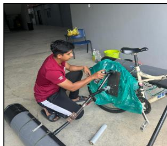
Figure 3.15: Repaint process to the steel surface
