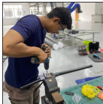
Figure 3.13: Drilling process of fold part
