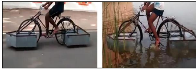
Figure 2.12 : Amphibious bicycle driving test on the road and inside the water
