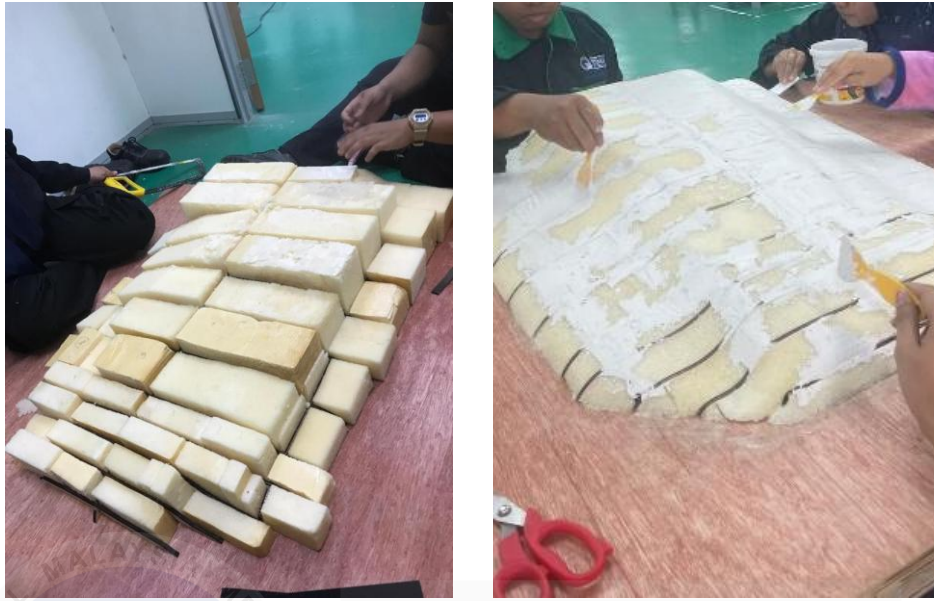
Figure 3.26 Rib and Spine Construction filled with high dense Polyurethane Foam.
