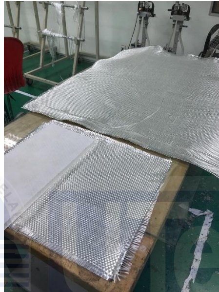
Figure 3.20 The materials used for all body parts (fibreglass cloth, GRP)
