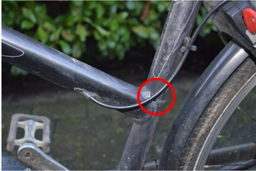
Figure 2.4 Fatigue crack in bicycle frame
