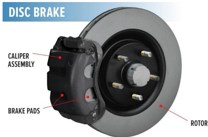
Figure 2.9 Disc Brake Components ( retrieved from WapCar.com,2024 )
