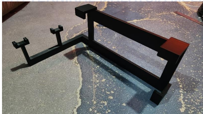
Figure 4.20 Brake Calliper Holder of Actual Prototype
