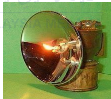
Figure 2.4: Figure show the system flame from rock and water (Carbide Lamps) (Source: Thorpe, 2005)
