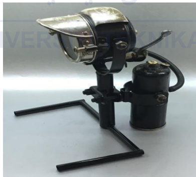
Figure 2.3: Carbide lighting for 1920's motorcycle (Source: Presscall, 2020)
