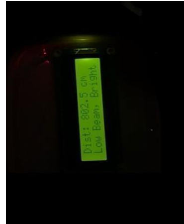
Figure 4.12: The LCD indicates that the area is bright, and the system switches to low beam.
