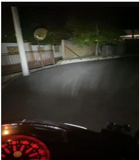
Figure 4.23: The image illustrates the system switching to high beam mode due to the absence of light detected by the LDR sensor.
