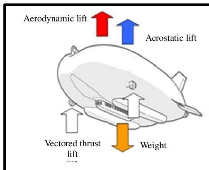
**Figure 2.3** Direction of Aerodynamic lift & Aerostatic lift (Prentice, 2014)
