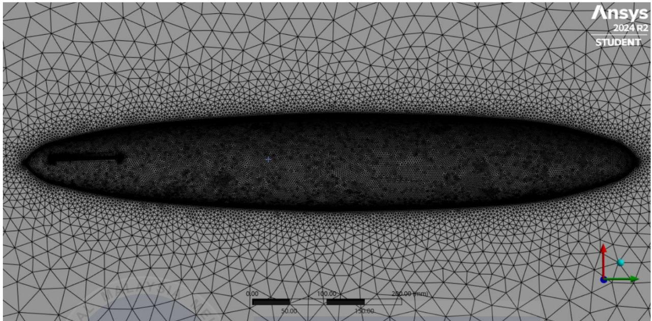
**Figure 4.1** Side view mesh of Blimps
