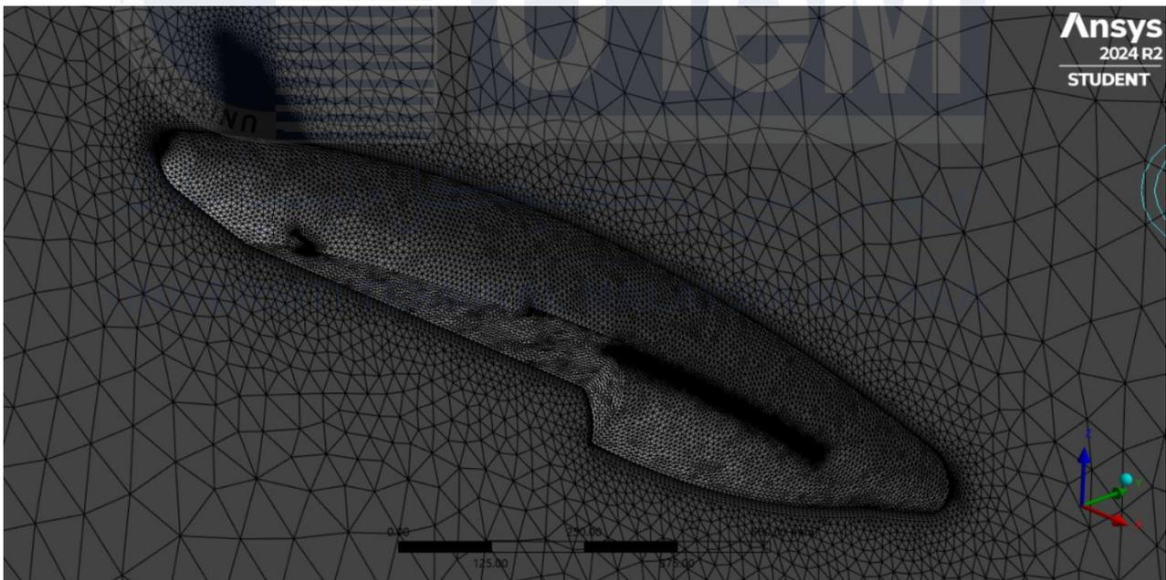
**Figure 4.4** 3D view mesh of RC Airship
