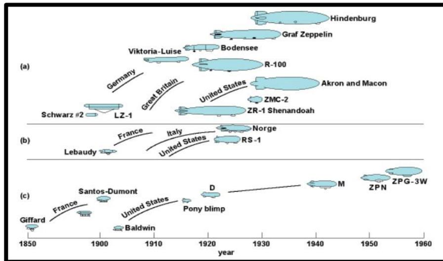
**Figure 2.1** History of Airship Development. (a) Rigid Airships. (b) Semi-rigid Airships. (c) Non-rigid Airships. (Stockbridge C, 2012)
