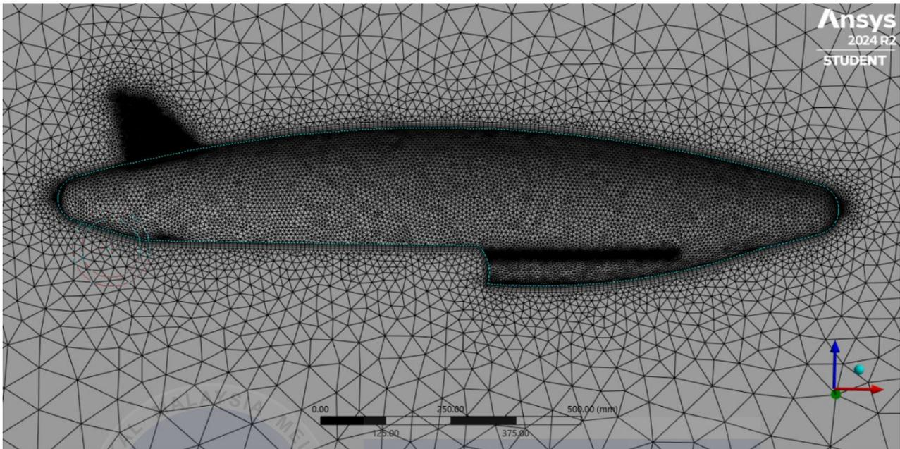
**Figure 4.3** Side view mesh of RC Airship
