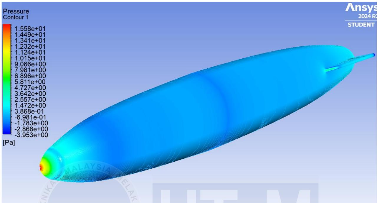
**Figure 4.5** Contour plot for Blimps
