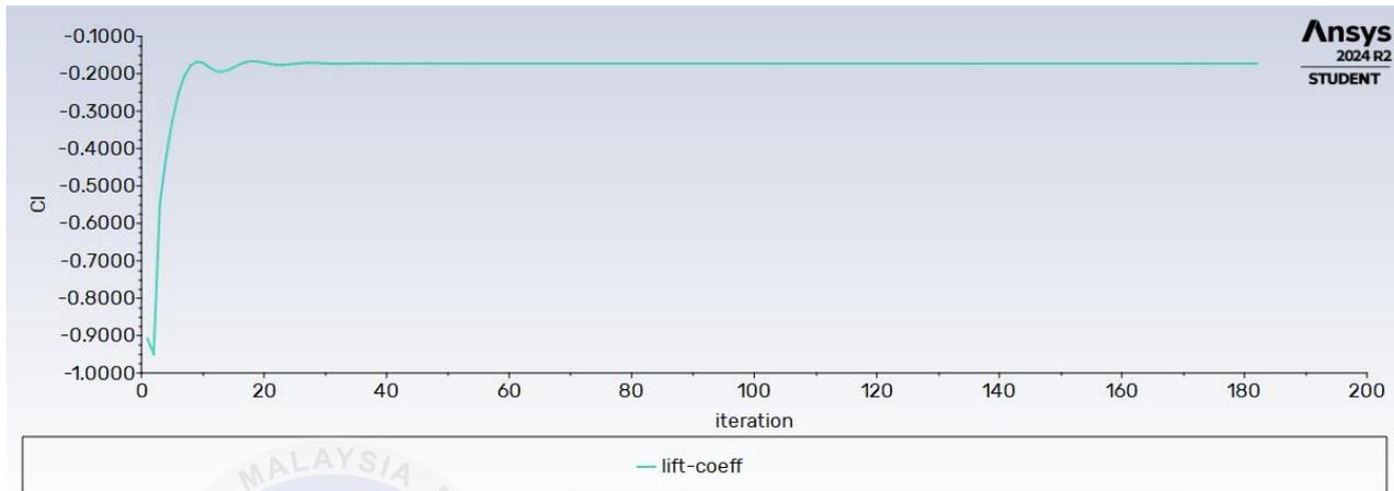
**Figure 4.9** Lift Coefficient of Blimps
