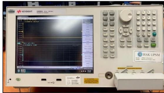
**Figure 3.7: E4990A Impedance Analyzer 20 Hz – 120 MHz**
