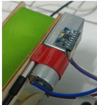
Figure 58: DS18B20 Temperature Sensor and MPU6050 Vibration Sensor Connected To The DC Motor
