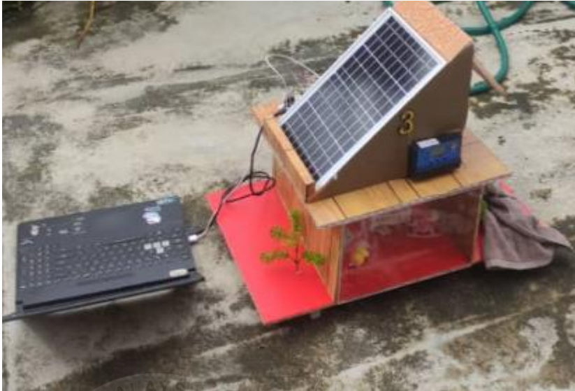
Figure 3-16 : Solar PV Data Collection Setup
