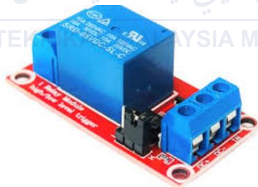
Figure 3-11 : Relay with 5V power
