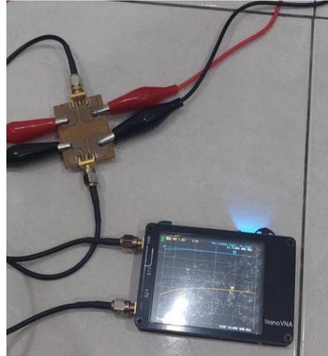
Figure 3.22 The setup connection of NanoVNA for seawater
