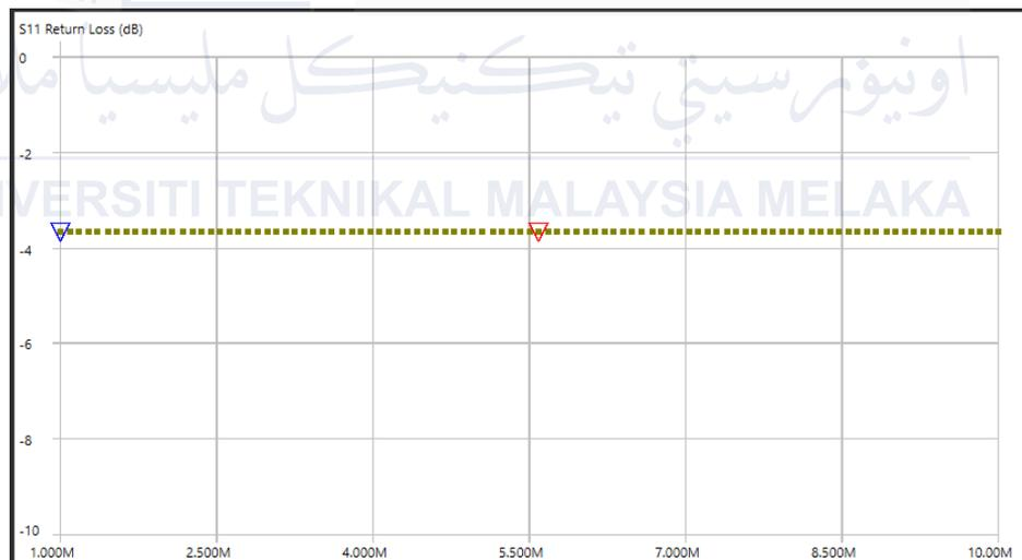
Figure 4.36 S11 Return Loss frequency response data captured by NanoVNA Saver in seawater
