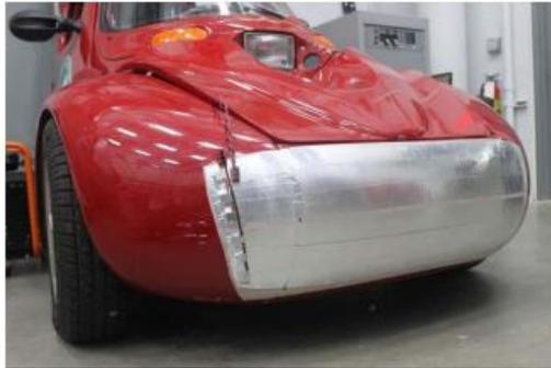
Figure 2.26 a) show conformal bumper charging station that has transmitter foil strips attached to a foam rubber [47].
