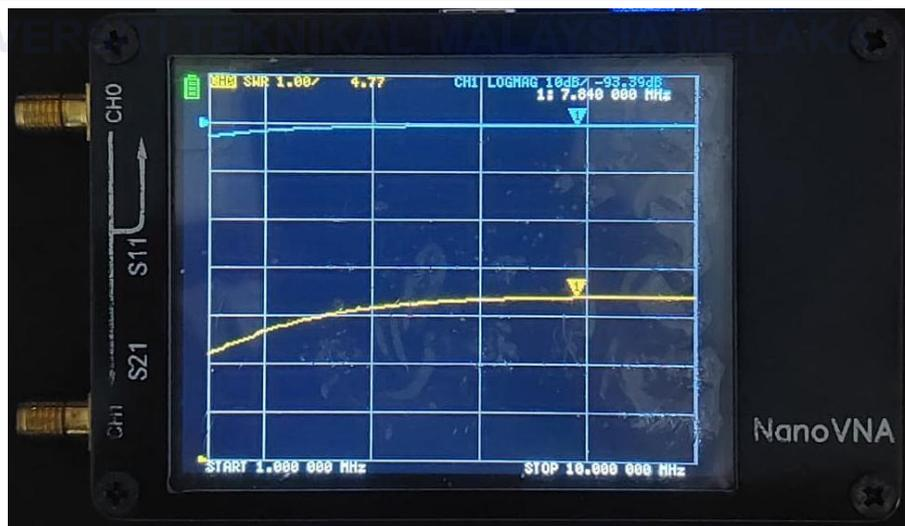
Figure 4.40 Frequency Response captured in Seawater using NanoVNA
