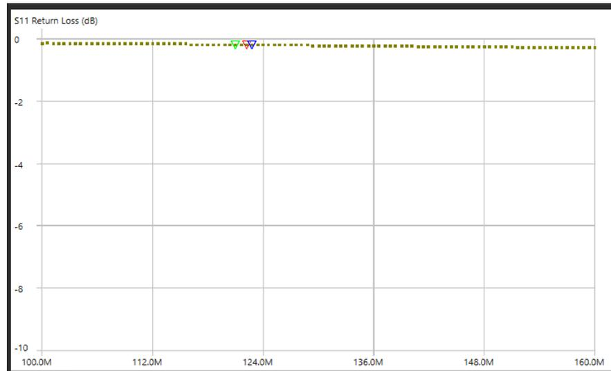
Figure 4.33 S11 Return Loss frequency response data captured by NanoVNA Saver in water.
