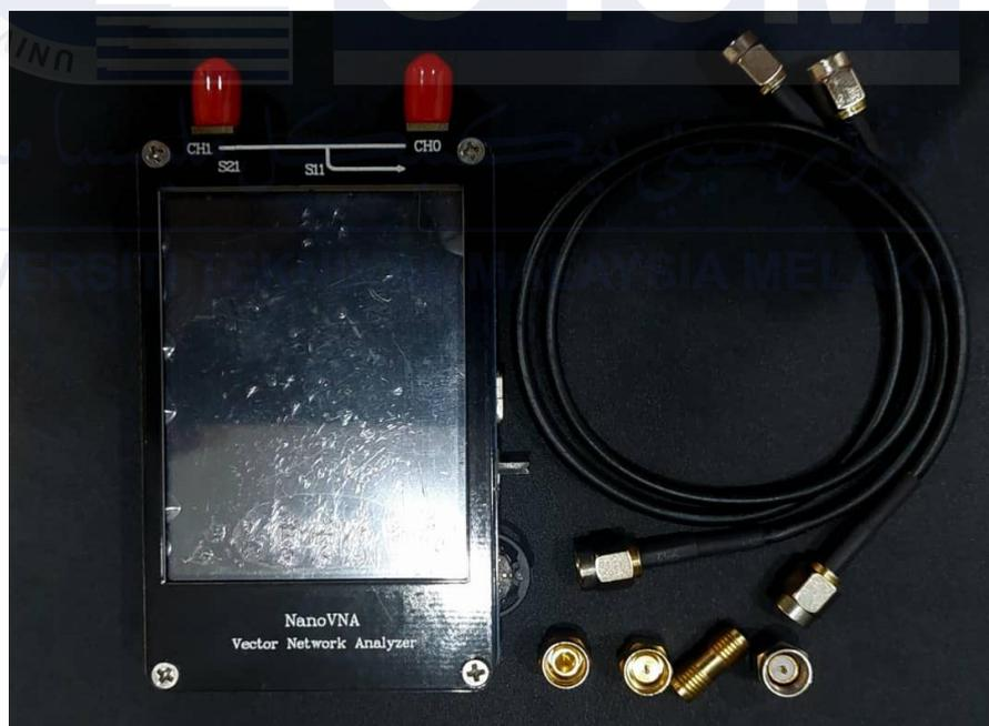
Figure 3.26 The NanoVNA vector network analyzer with its calibration standards for short, open and thru is used for accurate measurements.
