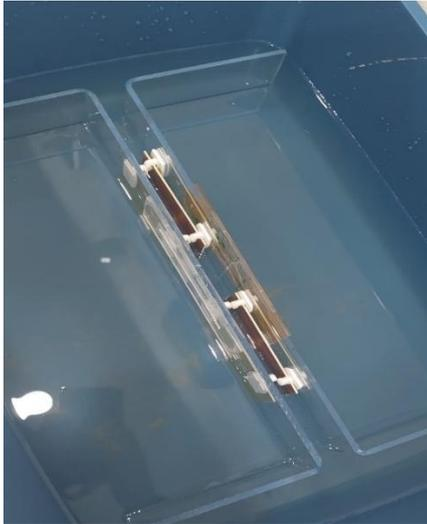
Figure 3.21 The condition of parallel plate in seawater
