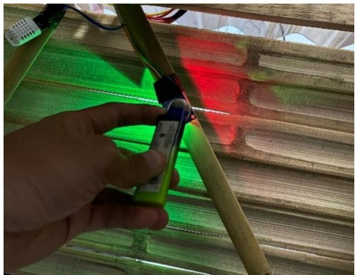
Figure 4.13 Butane gas is directed to the mq2 sensor
