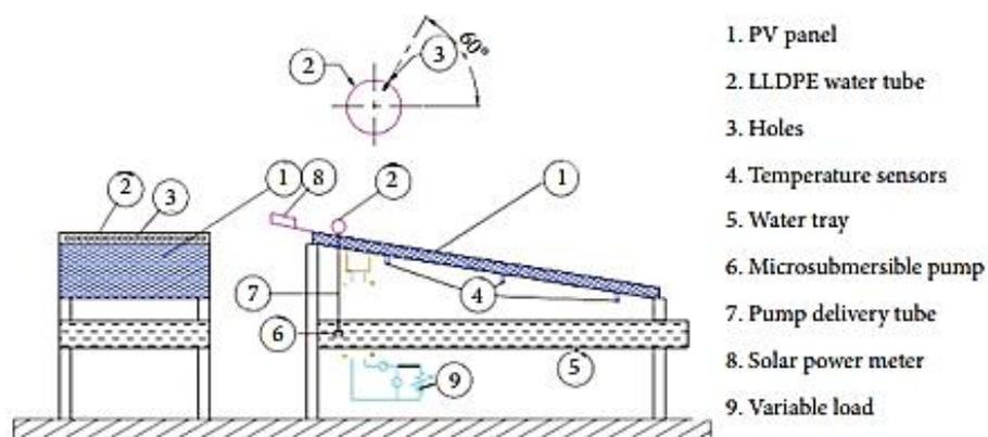
Figure 2.4 An active rear and front water cooling [14]
