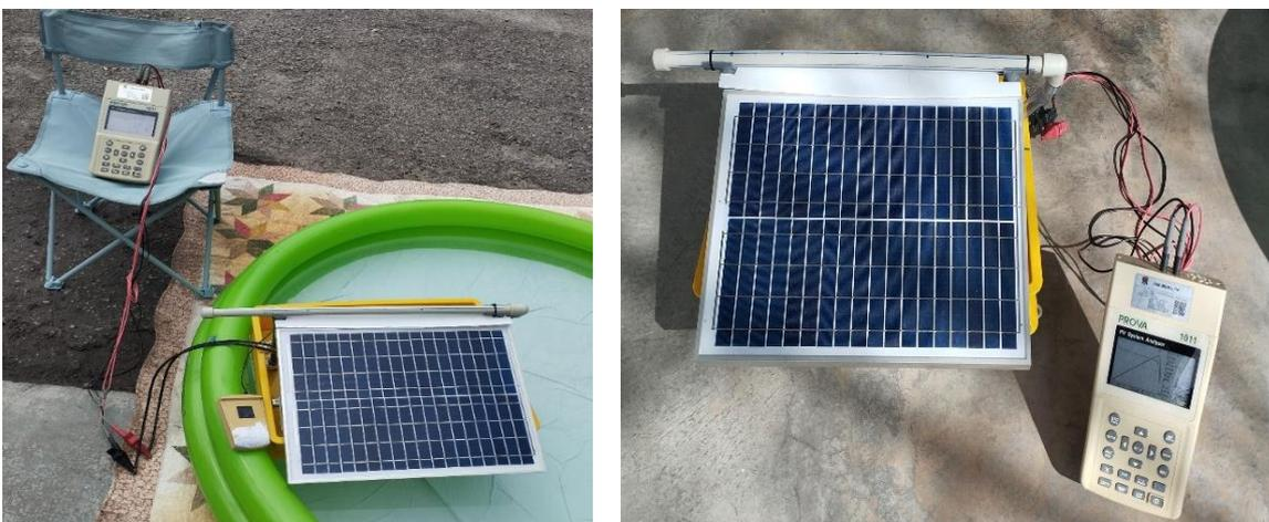
Figure 4.20 Data Collection Setup for *I-V* and *P-V* characteristics under real operating conditions
