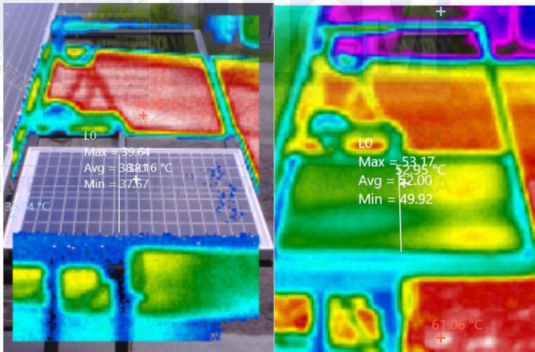
Figure 4.4 PV thermal images captured under real operating conditions
