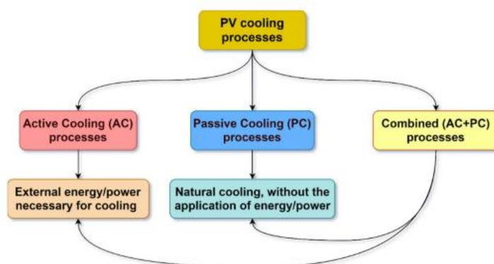
Figure 2.1 Classification of PV cooling processes
