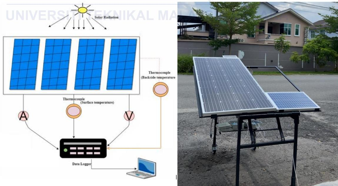
Figure 4.11 The experimental setup for data collection
