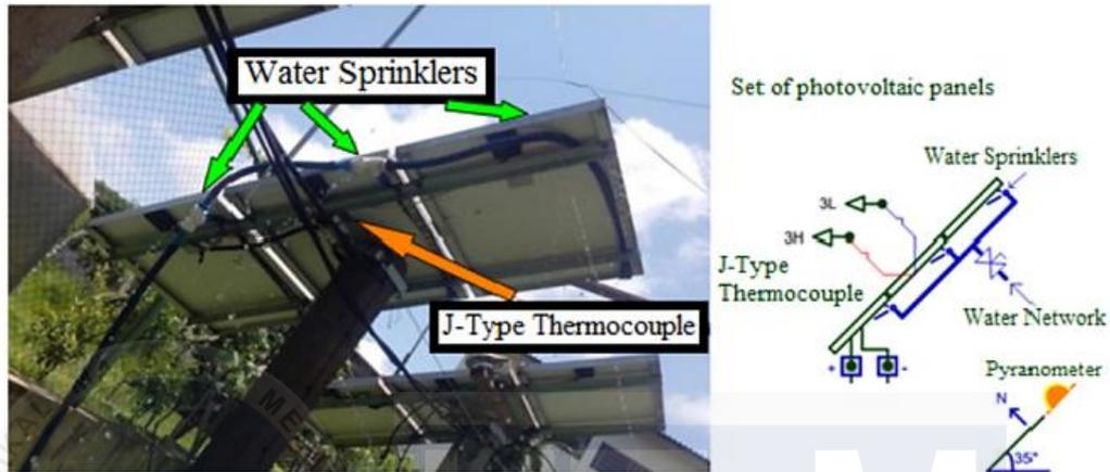
Figure 2.3 A photovoltaic panel with mounted water sprinklers [12]
