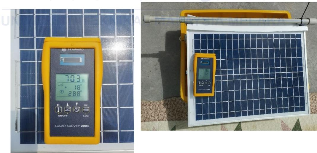
Figure 4.7 Tilt angle and irradiance measurement using SEAWARD Solar Survey 200R
