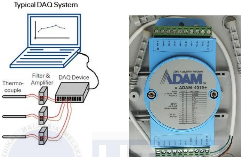
Figure 4.10 DAQ device and the setup
