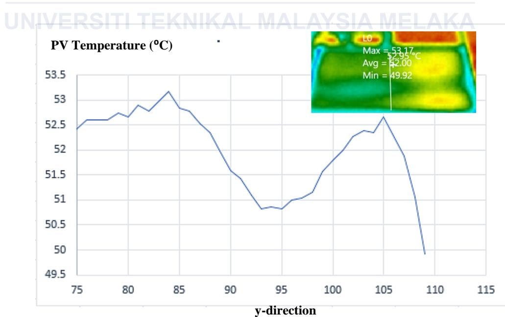
Figure 4.6 Temperature distribution across PV module at 558 W/m<sup>2</sup>
