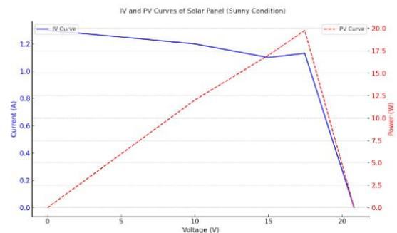
Graph 4-3 IV and PV Characteristics under Sunny Conditions
