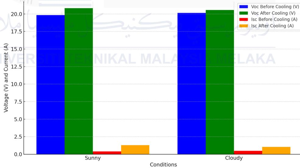
Figure 4.22 Comparative performance of voltage and current generated between cooling and without cooling implementation
