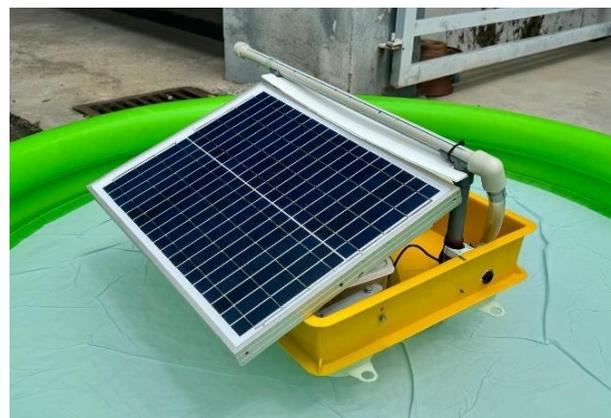
Figure 3.6 The developed prototype for floating PV with integrated cooling system
