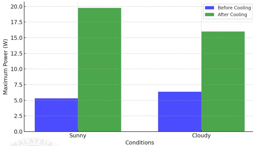
Figure 4.21 Comparative performance of maximum power generated between cooling and without cooling implementation
