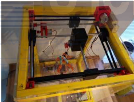
Figure 2.8 The construction of the X-axis and Y-axis movement [32]
